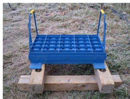
3 The amount of snow that is put into the Snowball-maker will be the right amount if you line up the table edge the Snowball-maker is on with the red line. Use the back of the scoop to hit the snow and shave it to get the right height. Also, remember to remove the excess snow that collects under the Snowball-maker so that more snow can fall off easily.
